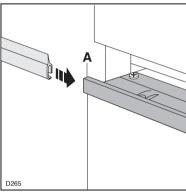
Open the door and push the appliance against the side of the kitchen unit opposite to that of appliance hinges.
